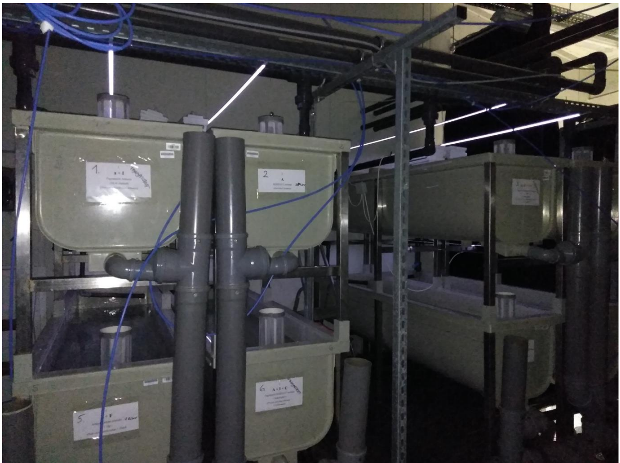
Fig. 2. RECIRK larval nursing system “valyus” applicable for sturgeons and catfishes.
