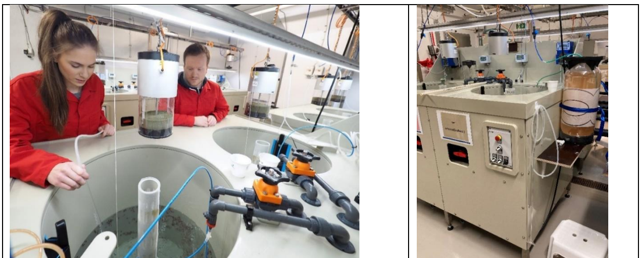
The CODTECH larval rearing laboratory is especially designed for experiments with fish larvae, plankton organisms, and fish juveniles. The tanks are “self-cleaning”, with fully controlled light, temperature, and water flow. Automated feeding is used for both live prey and formulated diets. There are 16 self-cleaning rearing tanks (á 100-200 L) available in this laboratory.
