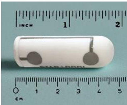
Figure 4. STAR ODDI data logger for heart rate, activity and temperature measurement ( https://www.star-oddi.com/products/archival-tags/animal-heart-rate-activity-logger )
