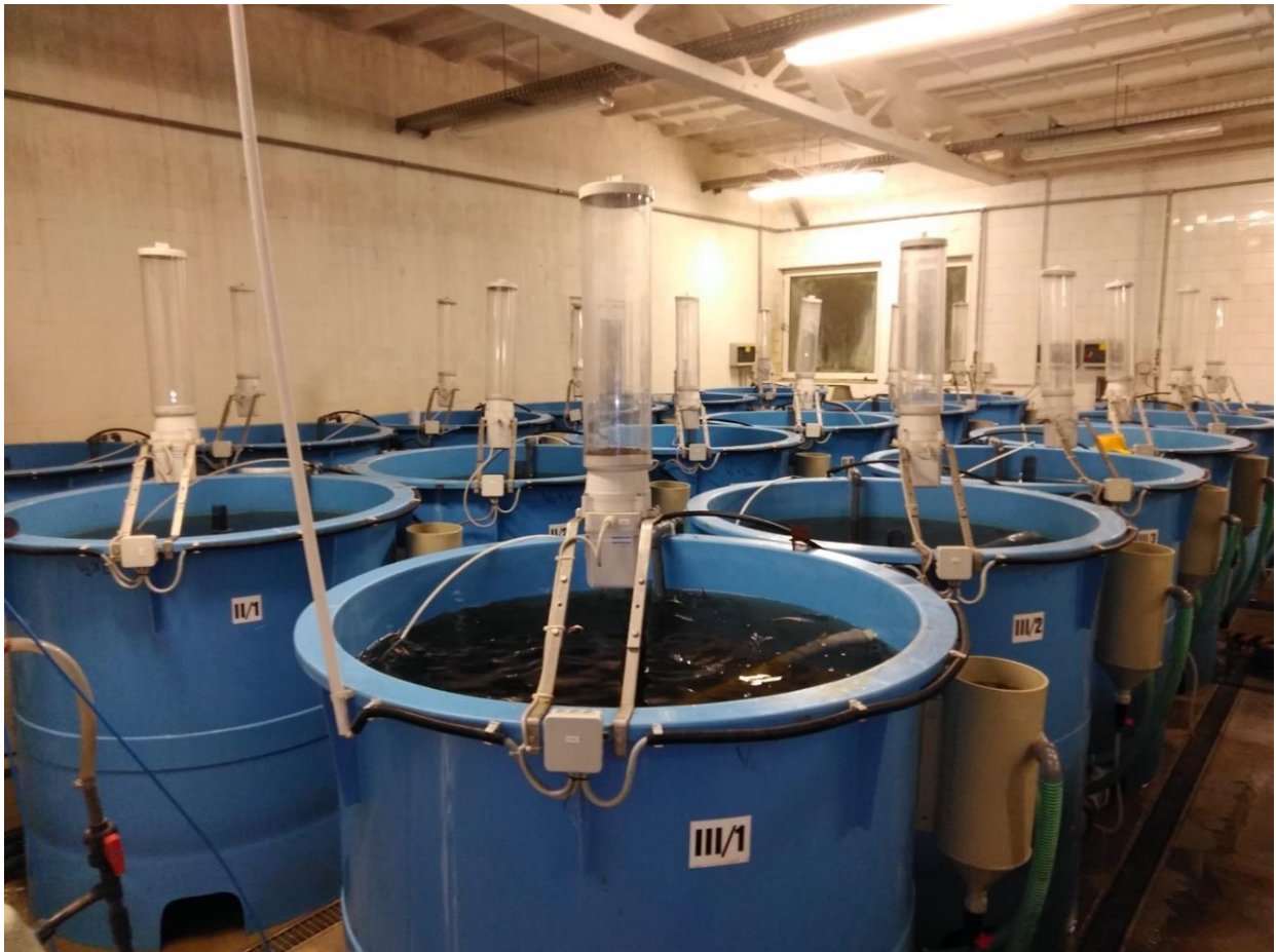
Fig. 3. RECIRK “18-as” system composed of three identical independent RAS units.
