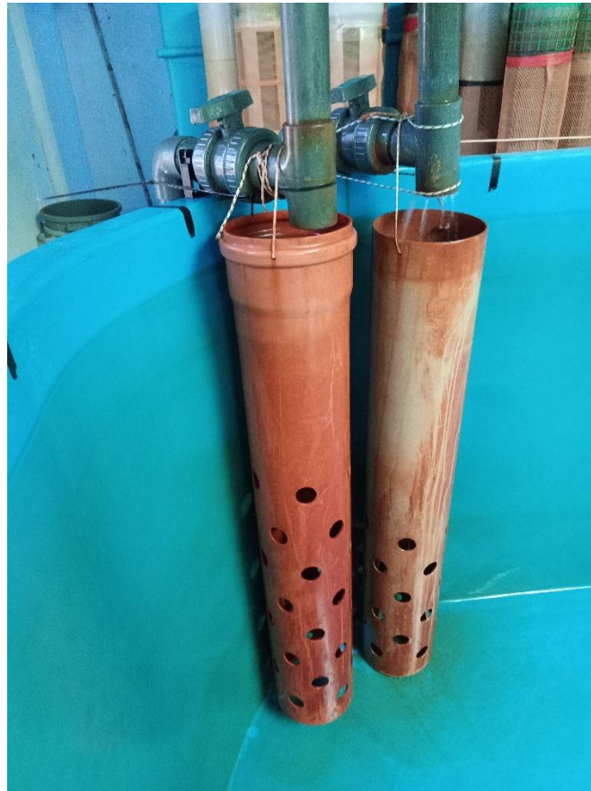
Figure 10: Photograph of the HCMR tank with the inlet arrangement using a current reduction device.
